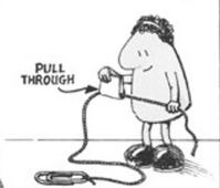
c. Slide the thread through the tape until you find a length where your pendulum swings exactly one cycle each second.
